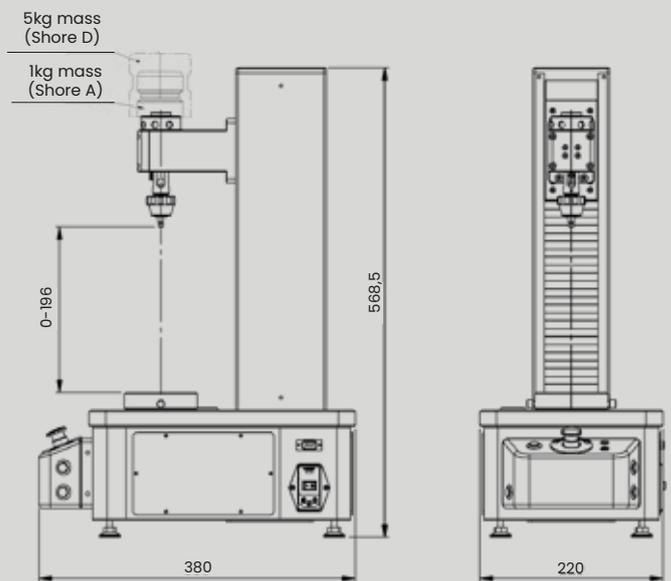
Possibility of adding a calibrated mass for all Shore scales on one instrument
