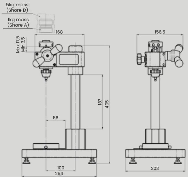
Possibility of adding a calibrated mass for all Shore scales on one instrument
